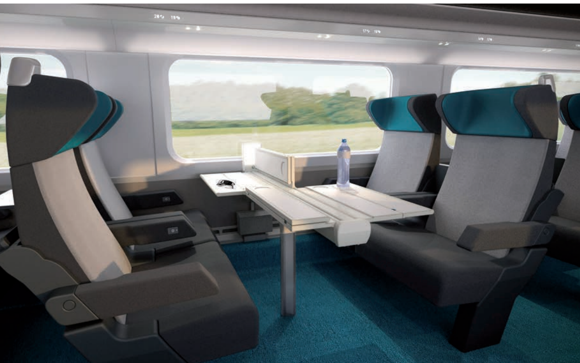
The new 'portfolio' table & special grab bar for PRM (below) make for ease of movement
